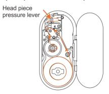
• Close the paper roll press block, tighten the paper winding shaft, screw the head piece pressure lever, close the side cover of printer, Long press the FEED button until the light flashes and then let go.
