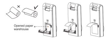
Open the side cover, remove the paper roll press block
