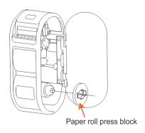
Unscrew the head piece pressure lever and load paper as shown in the figure.(There are decorative paper tips in the module)
